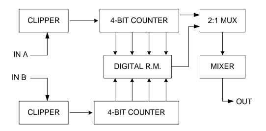
The "heart" of the MOTM-120 are the two 4-bit counters, which are 74HC161s (U1 and U2). The counters have a *clock input* (pin 2) that causes the 4 outputs to increment, in a binary fashion, from 0 to 15, then repeat. The 4 outputs are as follows:
