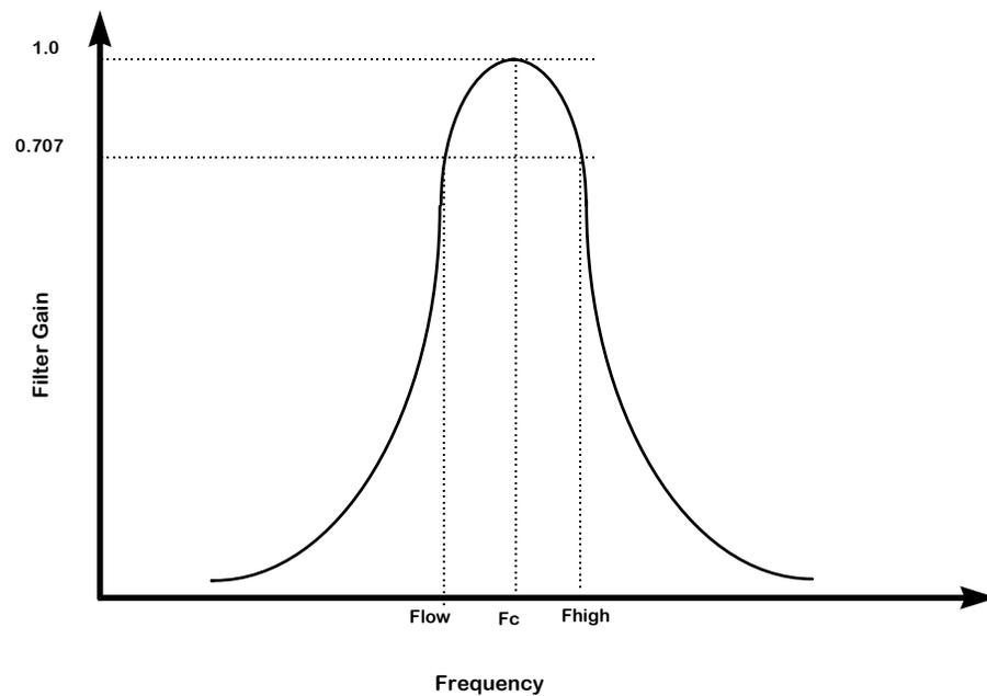
For example: if our filter is tuned to 1000Hz, the input audio is attenuated by 3dB (a factor of 0.7) at 900Hz and 1100Hz. Bandpass filters do not have a “slope” associated with LP and HP filters.
