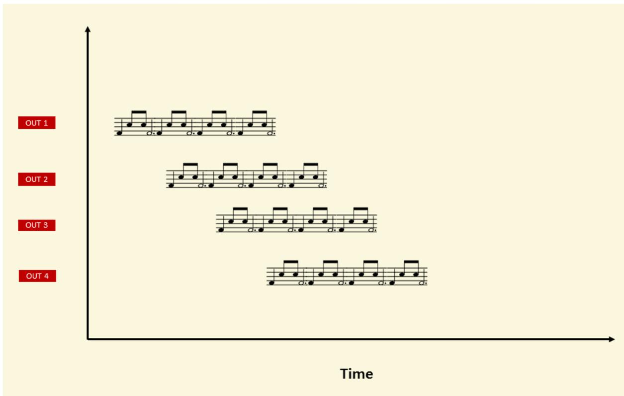
The diagrams of these notes imply different note lengths, but in reality the note ‘duration’ is the period of the clock. If the internal clock is used, then all the notes generated are of equal length. The circuitry in the E102 samples the INPUT CV and updates all 4 OUT jacks only when there is a rising edge of the clock. The clock can be a LFO, the Trigger out of a drum machine, or even an Envelope. Remember, the period/frequency of the clock sets the note “on time”, not the clock’s duty cycle.
