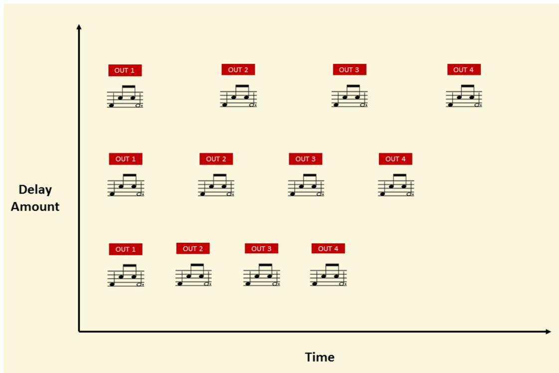
Notice how the sequence of notes is repeated in time sequentially on the four outputs. By increasing the amount of DELAY between the stages, it takes a larger amount of time for the sequence to be outputted from each stage. Remember that the E102 and the CV sequencer use the same clock source, so the RATE of the clock is constant. This allows for the time relationship between the notes of the sequence to remain identical regardless of the amount of applied DELAY.
