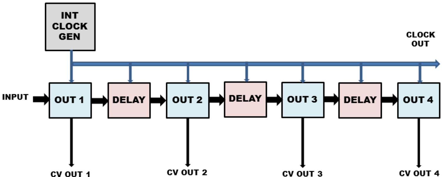
Figure 1: Simplified Block Diagram
